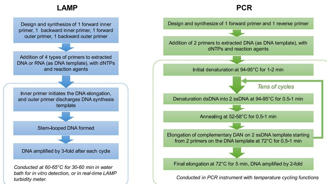
**Fig. 2.** Comparison of LAMP and PCR processes. Further, for real-time quantitative PCR, DNA probes with one-end of quencher and one-end of fluorescent dye are added. For RNA detection in PCR, complementary DNA of the RNA shall be synthesized. For one-step RNA-PCR reaction, enzyme will be further added in PCR reaction tube.
