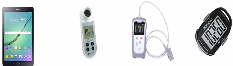
FIGURE 5 Telerehabilitation. Patients monitor vital signs using Bluetooth-enabled wearable monitors that transmit data to a cloud-based platform via an application installed onto the tablet. Health professionals can log in and see if the patient has uploaded data, and provide feedback [145].
