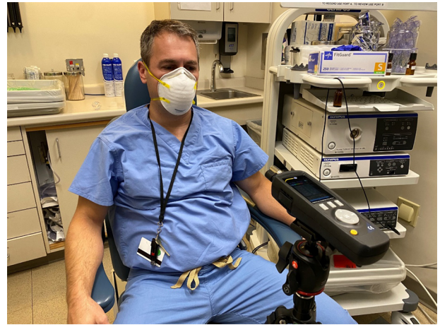
Figure 2. Participant sitting upright in clinical examination room chair 16 in from the intake port on particle counter.
