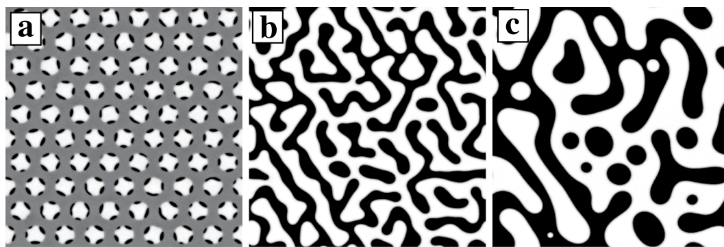
Figure 7. Time evolution of the dendritic pattern with multiple propagated triggers when \Delta d = 60 , \bar{\phi} = 0.1 , and v_{tri} = 0.01 . (a) By t = 3500 , a dendritic pattern has formed at each core. (b) At t = 50000 , a connected pattern is observed. (c) The same can be seen when t = 100000 . Connectivity can be seen for a long time despite the fact that \bar{\phi} = 0.1 .
