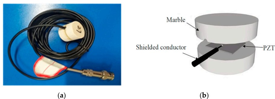
Figure 1. The embeddable piezoceramic smart aggregate. (a) The photo of a piezoceramic smart aggregate; (b) Three-dimensional schematic of a piezoceramic smart aggregate.
