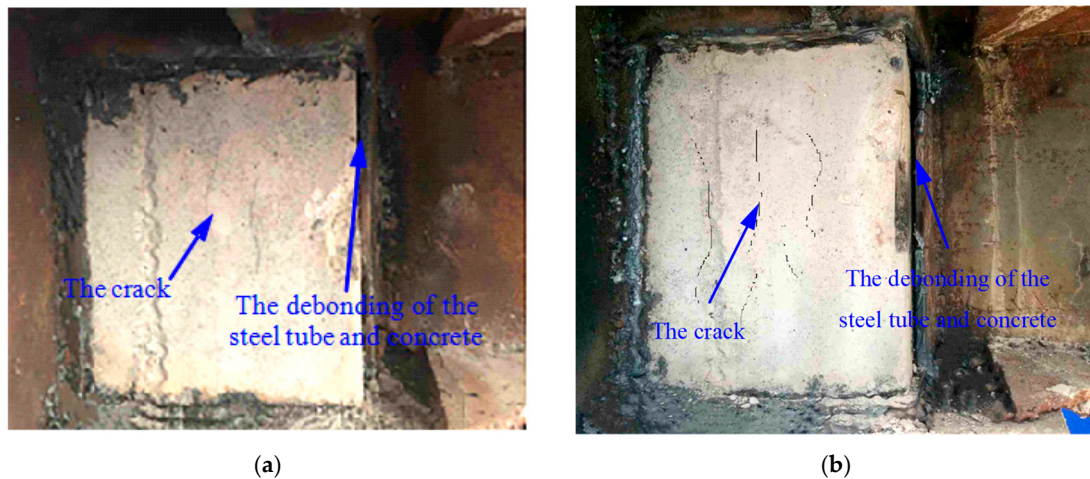
Figure 11. Damages to the joint specimens (cut-away view). (a) Specimen JD-1; (b) Specimen JD-2.
