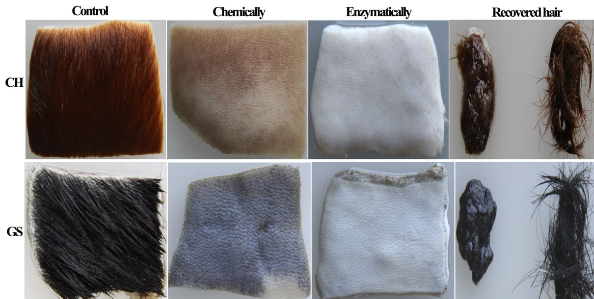
Figure 7. Dehairing effect by conventional chemical treatment versus enzymatic method with crude AprA-PPC. CH represents cattle hide; GS represents goat skin. The dehairing treatment was performed at 40 °C for 10–12 h. In the picture of recovered hair, chemical dehairing result is shown in the left, whereas enzymatic dehairing result is shown in the right.
