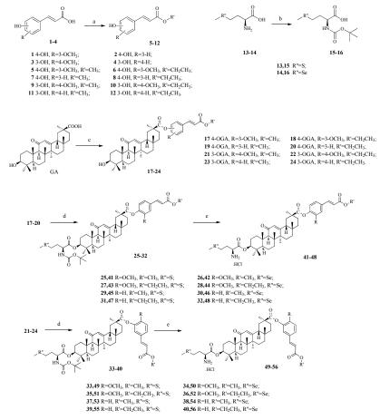
*Reagents and conditions*: (a) CH<sub>3</sub>OH or CH<sub>2</sub>CH<sub>3</sub>OH, H<sub>2</sub>SO<sub>4</sub>, reflux; (b) 1,4-dioxane-H<sub>2</sub>O, NaHCO<sub>3</sub>, (Boc)<sub>2</sub>O, rt; (c) ferulic acid analogs, EDCI, DMAP, CH<sub>2</sub>Cl<sub>2</sub>, rt; (d) Boc-L-methionine or Boc-L-selenomethionine, EDCI, DMAP, CH<sub>2</sub>Cl<sub>2</sub>, rt; (e) HCl<sub>(g)</sub> in CH<sub>2</sub>Cl<sub>2</sub>, rt.
