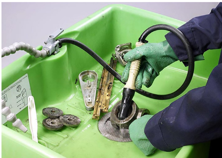
FIGURE 15.2 Cleaning of parts in a wash basin [33]. (Courtesy of J. Walter Co. Ltd, Quebec, Canada).
