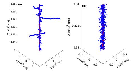
**Figure 5.** A representative track structure for a 5 MeV proton at the entrance part (**a**) and in the Bragg peak region (**b**). The proton was emitted along the positive *Z* direction. Red and blue dots represent the energy depositions by the proton and secondary electrons, respectively. Note: in the two subplots, we kept the same aspect ratio between the *z* and x/y axes, but plotted them with different ranges.
