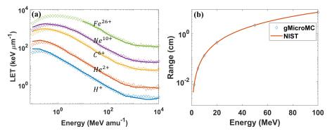
**Figure 2.** (a) The unrestricted LETs for different ions with different energies. The unit  $amu^{-1}$  means per nucleon. Solid lines represent data extracted from Plante et al.'s work, while data with diamond symbols are from our simulation with gMicroMC. (b) The simulated proton range for different energies.
