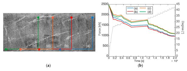
**Figure 16.** (a) Evaluated areas for HPZ04, and (b) Rotation of the principal strain direction during loading for HPZ04.
