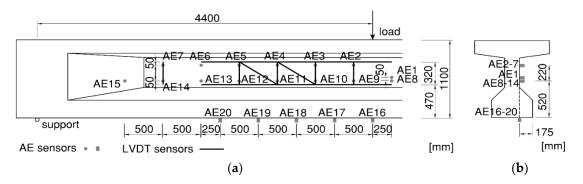
Figure 3. Sensor plan for beam HPZ04 showing LVDTs and AE sensors: (a) Side view; (b) cross-section.
