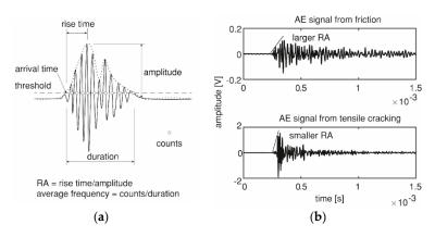
Figure 5. (a) Illustration of AE parameters and (b) AE signals from friction and tensile cracking.
