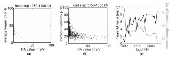
**Figure 14.** (**a**,**b**): Average frequency and RA value of each AE event at load steps 1050–1100 kN and 1750–1800 kN, respectively, and (**c**): Changing of mean average frequency and mean RA value with loading.
