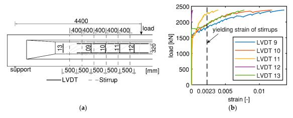
**Figure 10.** Measurement of yielding stirrups from LVDTs for HPZ04: (**a**) Position of the stirrups and LVDTs; and (**b**) Vertical deformation results of LVDTs.
