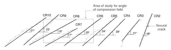
Figure 17. Crack pattern and crack angle from DIC results of HPZ04.
