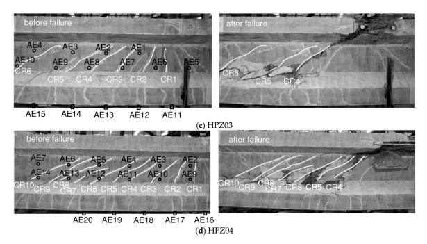
**Figure 11.** Crack patterns in the four girders from DIC results before and after failure, with the locations of AE sensors: (a) HPZ01, (b) HPZ02, (c) HPZ03, (d) HPZ04.
