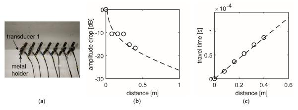
Figure 4. Baseline measurement in HPZ03: (a) Setup, (b) amplitude drop, and (c) wave speed.
