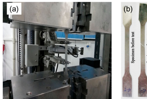
Figure 3. Tensile test of the materials: (a) equipment, and (b) specimens for tensile tests.
