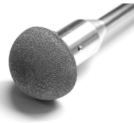
Figure 3. Photograph of the Ti acetabular cup surface finish created in a single part (i.e., no coating) by powder bed fusion additive manufacture on a Renishaw AM250 machine. [Correction added on 08 August 2019; Figure 3 legend was corrected]
