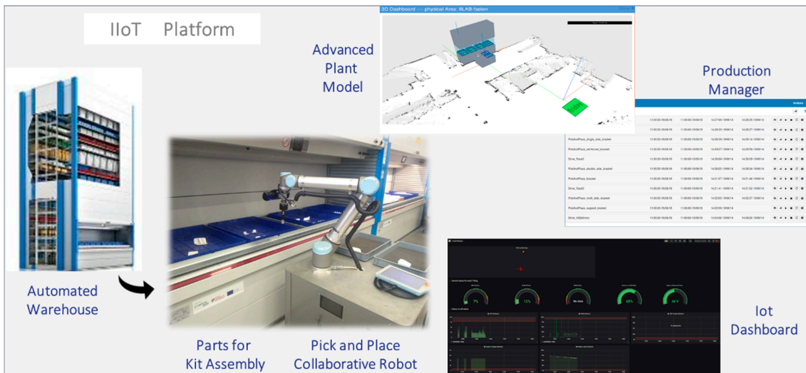
Figure 11. Main components of the adaptive pick and place robot in the logistics warehouse.
