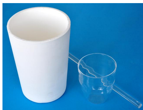
Figure 6. Crucibles applied in the glass melting processes: 1100 cm 3 in volume made of ground and sintered quartz glass; 200 cm 3 in volume made of clear quartz glass; 10 mm in diameter quartz glass rod used for glass melt stirring.
