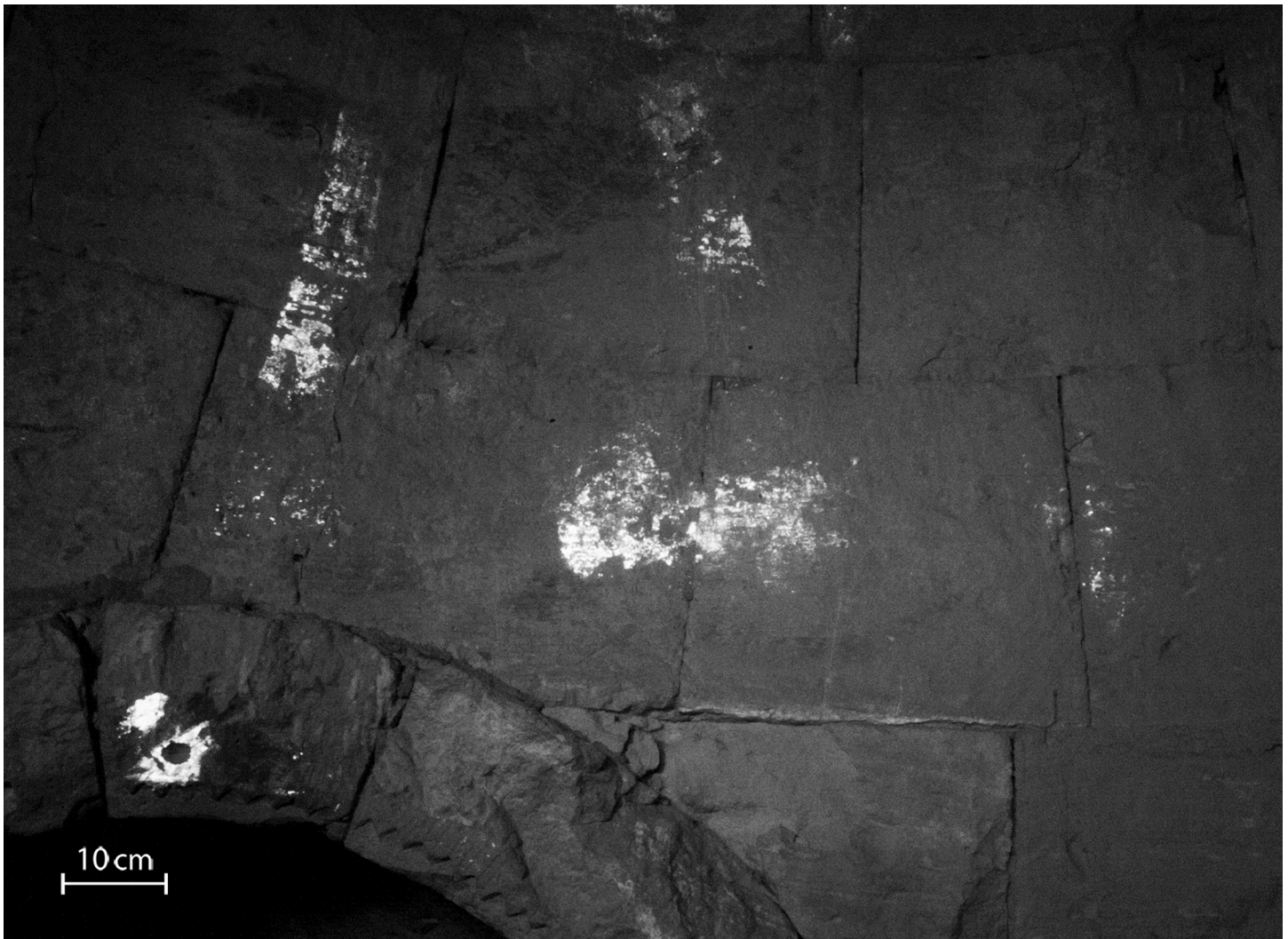
Fig 5. VIL image of the lower right part of the Transfiguration wall painting. The image shows the intense emission of areas painted with Egyptian blue, which appear in very bright white (Photo: R. Linn, 2016).
