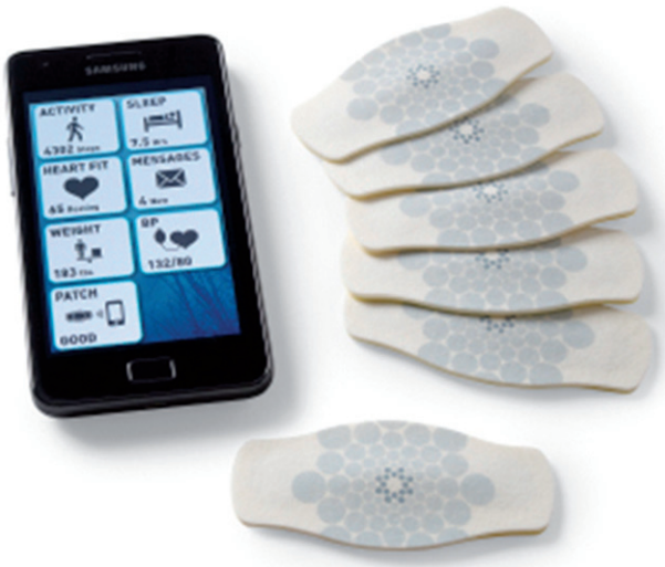
Figure 1. Adhesive activity and heart rate monitoring patch used in the study (Proteus Digital Health, Redwood City, CA).
