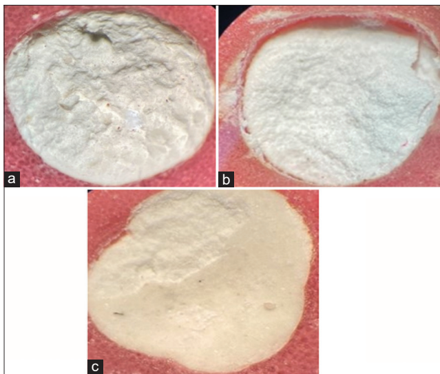
Figure 1: (a) Stereomicroscopic imaging showing cohesive failure, (b) Stereomicroscopic imaging showing adhesive failure, (c) Stereomicroscopic imaging showing mixed failure
