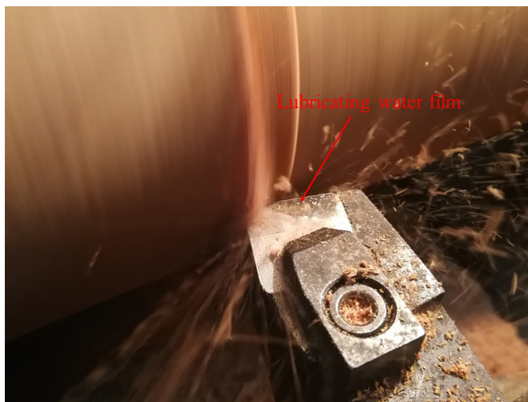
Fig 17. Forming lubricating film with seeped free water.
