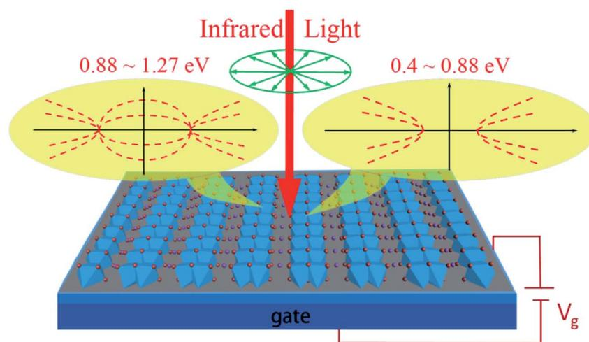
Fig. 5 Schematic diagram of the gate tunable NIR hyperbolic device by FETs. When a NIR incident light illuminated on monolayer  $\text{NaW}_2\text{O}_2\text{Br}_6$ , the propagation behaviors of NIR light in monolayer  $\text{NaW}_2\text{O}_2\text{Br}_6$ , including the propagation direction, the FoM, and even the topology (depending on the wavelength of NIR light), can be manipulated by the gate voltage.
