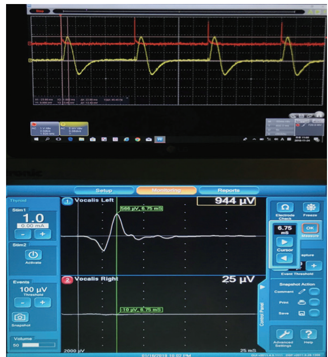
Fig. 2. Electromyography (EMG) and endotracheal tube with pressure sensor recordings, showing the amplitude and latency of EMG and the pressure sensor for 1 mA stimulation using the Nerve Integrity Monitor 3.0 system in pig. Upper graph, pressure sensor signal; Lower graph, EMG signal.
