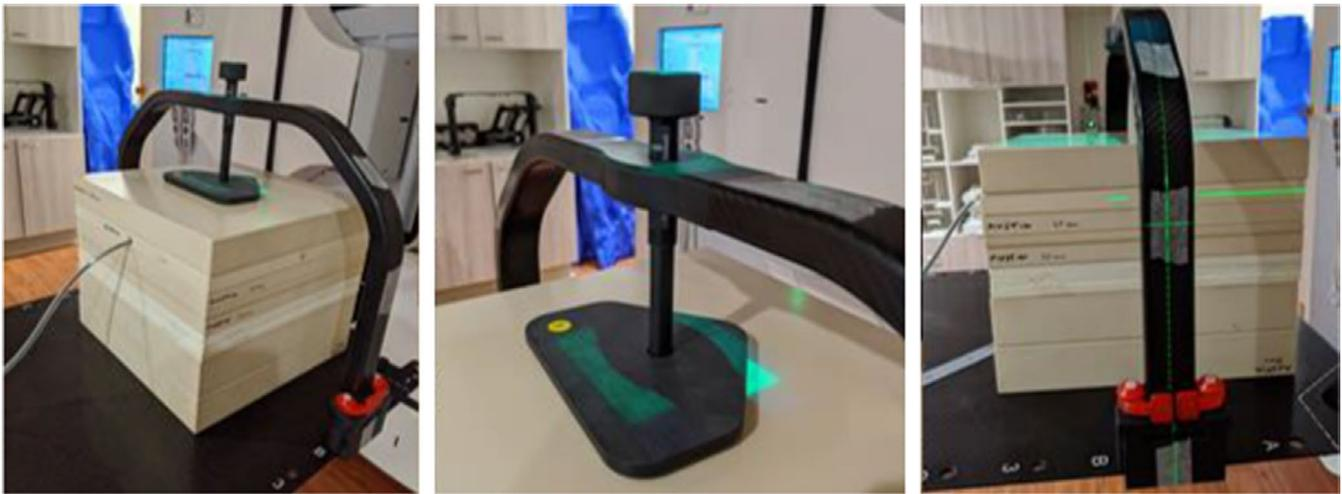
**FIGURE 3** Phantom and device setup on the linac for measurement
