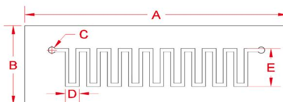
**Fig. 1.** AutoCAD design for PMMA pre-recorded sheet. A - Sheet length 75 mm, B - Sheet width 25 mm, C - In and out diameters 2 mm, D - Horizontal trajectory 4 mm, E - Vertical trajectory 12 mm. The design has a total linear trajectory of 292 mm and a channel width of 1 mm.
