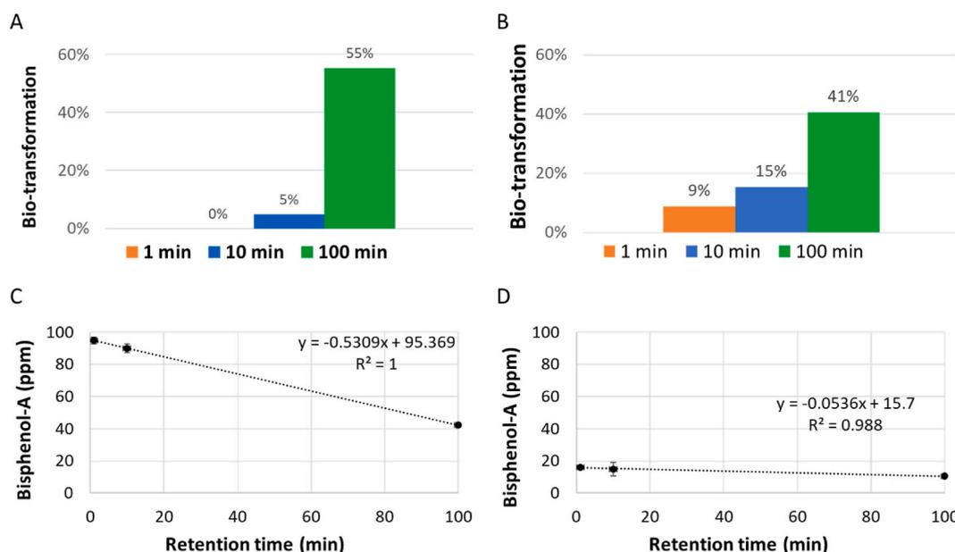
**Fig. 4.** Final bisphenol A (BPA) transformation percentage at retention times of 1, 10, and 100 min with an initial concentration of A) 100 ppm., and B) 20 ppm. Bisphenol A (BPA) transformation at 1, 10, and 100 min retention times with an initial concentration of C) 100 ppm., and D) 20 ppm.
