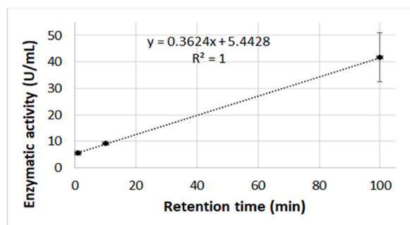
Fig. 3. ABTS oxidation in the biocatalytic reactor of enzymes immobilized with EDC.
