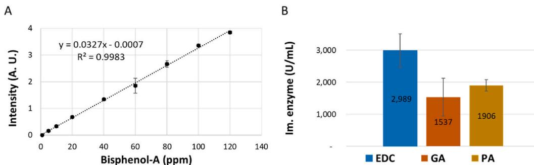
**Fig. 2.** A) Standard curve obtained for the Bisphenol A quantification. B) Enzyme immobilization through the different cross-linking agents EDC, and GA contrasted with passive immobilization method (PA).
