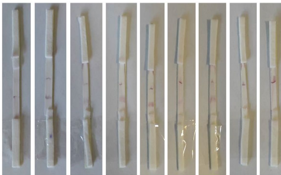
Figure 5: Images form LFTSs upon loading with different samples when they prepared at optimized conditions. 7 left samples are positive, and 2 right samples are negative.
