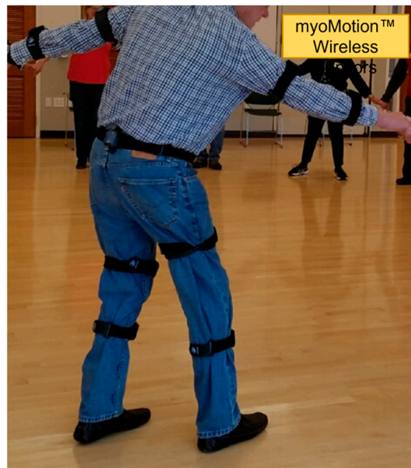
Figure 1. Dance students wore the Noraxon myoMOTION™ devices for a one-hour long session. These devices were attached to the arm, forearm, hip, thigh, and leg, and activated during each dance practice.
