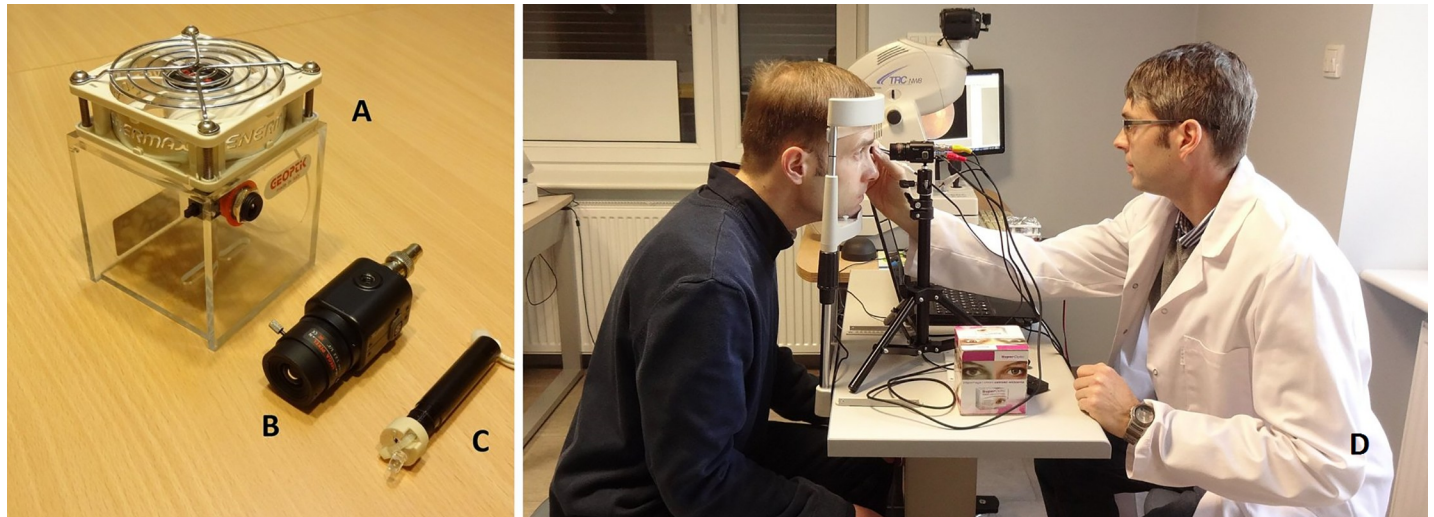
Fig 1. Main components of prototype apparatus. A—cooling fan. B—camera with lens. C—near-infrared transilluminator. D—near-infrared iris transillumination examination conducted by the author.
