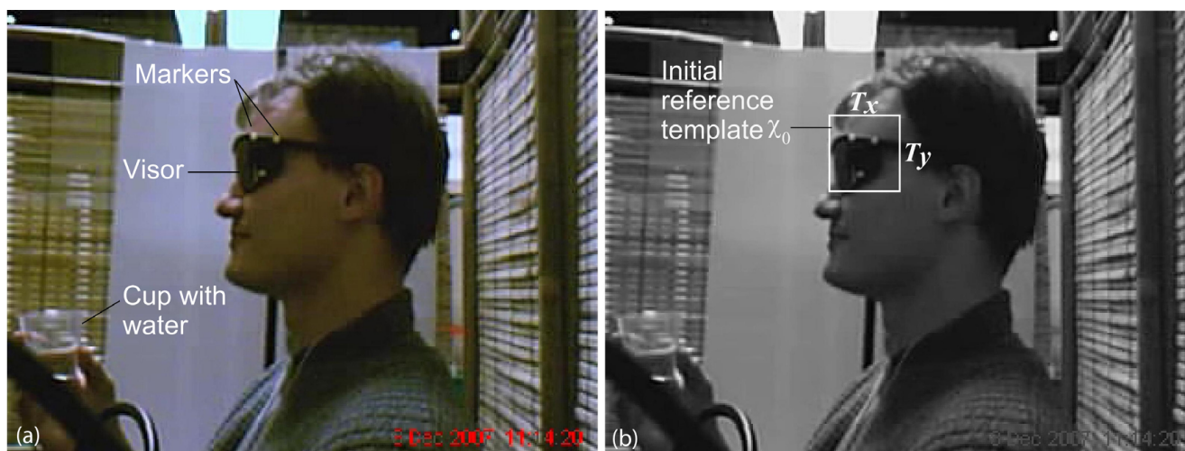
Figure 2 Data acquisition approach and marking of the initial reference template. The acquired data: (a) a participant wearing the standard-issue visor with markers; (b) the initial reference template for tracking head position.
