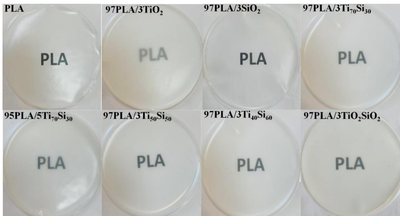
Figure 9. Photographs of films prepared from PLA, PLA/TiO 2 , PLA/SiO 2 , PLA/Ti x Si y , and PLA/TiO 2 SiO 2 composites ( 250 \pm 4.68 \mu\text{m} thickness).
