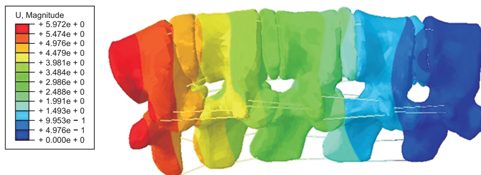
Fig. 4. Relative displacements of intervertebral discs (mm) under 45% of body weight loading.
