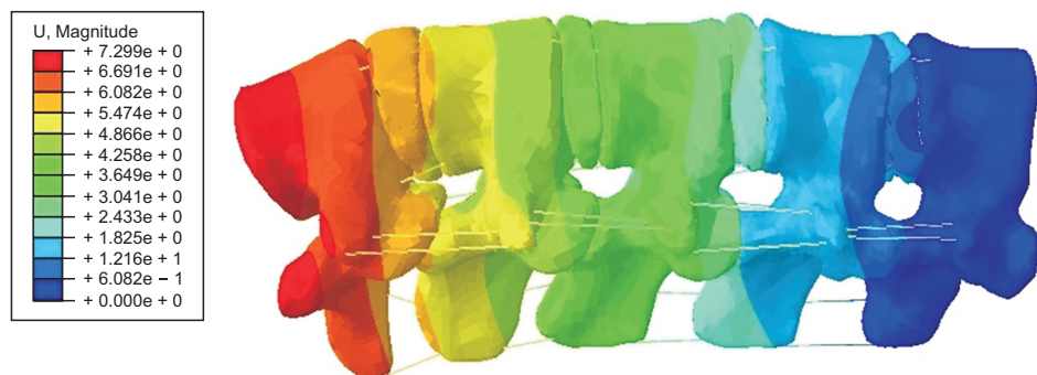
Fig. 5. Relative displacements of intervertebral discs (mm) under 55% of body weight loading.
