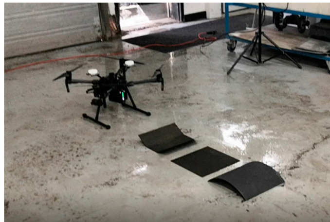
Figure 2. Image of the UAV along with the specimen for the first experimental setup.
