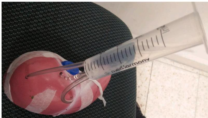
**Fig. 4.** The construction of the input part; three tubes connect to the large syringe.
