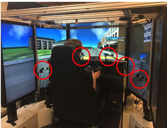
Figure 1. Image of the driving simulator equipped with six cameras (red circles, with the last camera obstructed from view by the chair) located around the driver's seat (2 on the left, 2 on the right, and 2 in the center), which enabled recording of lateral eye and head position up to 90 degrees to the left and right of the driver.
