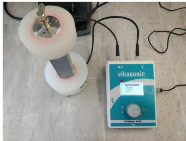
Figure 3. Measurement of the dynamic elastic modulus.
