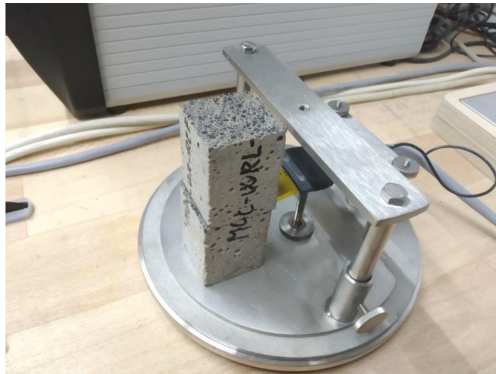
Figure 4. Experimental setup for thermophysical parameter measurement.
