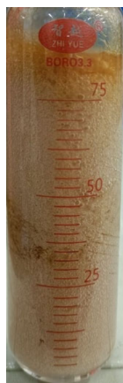
Figure 1. Subsequent colloidal state of gel foam at high temperature and high salinity.
