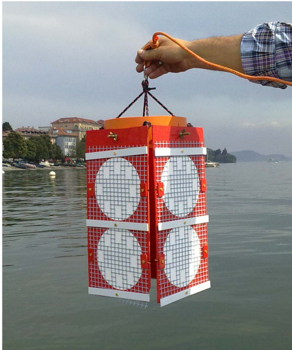
Figure 1. Device used for artificial substrate suspension in Lake Maggiore.
