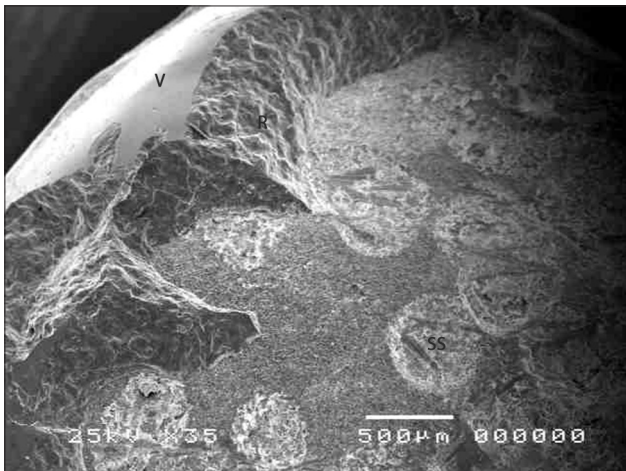
Figure 3: Veneer debonding: Spot size (SS) of about 0.5 mm corresponding approximately to the diameter of the laser sapphire tip
