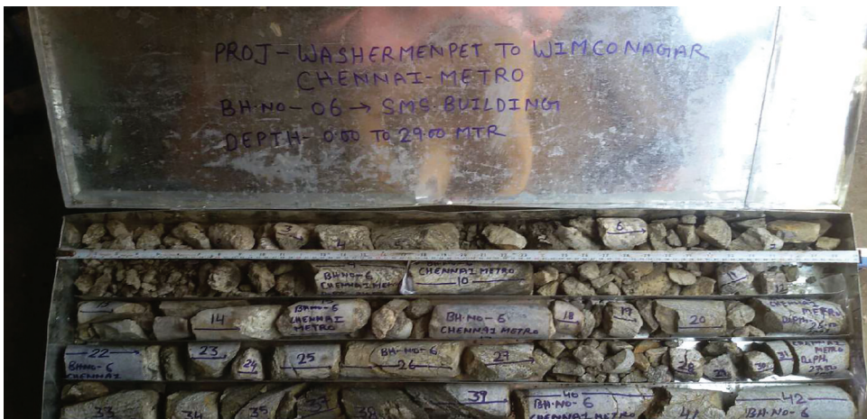
FIGURE 7 Box of core samples from Washermanpet survey. From CMRL tender documents.
