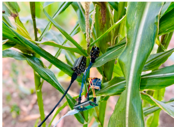
Fig. 1. VOC and Ultrasound sensors on planted maize crops.
