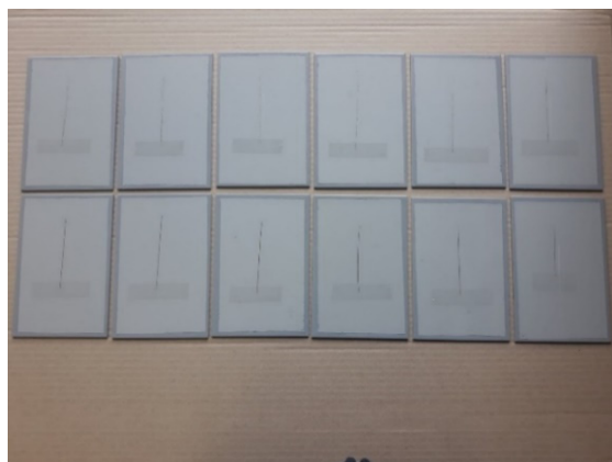
Figure 4. Prepared specimens before being placed in the salt-spray test chamber.
