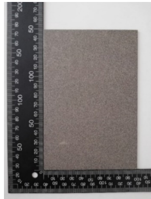
Figure 2. Test sample after abrasive jet treatment.
