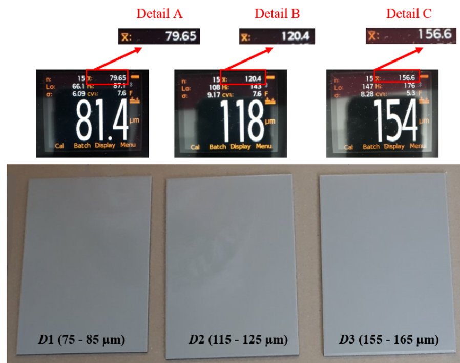
Figure 3. Test specimens after coating.
