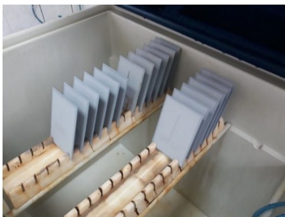
Figure 5. Test specimens inside the salt chamber workspace.
