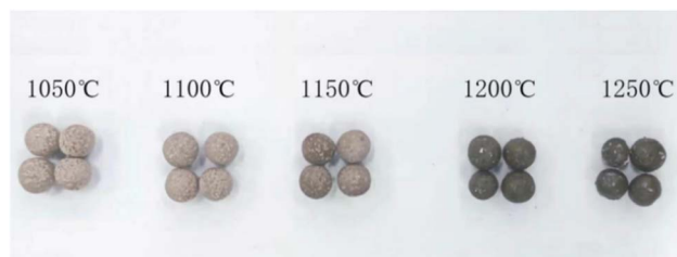
Fig. 12 Morphology of ceramsite at different sintering temperatures.
