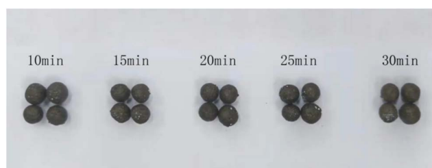
Fig. 15 Morphology of ceramsite at different sintering time.
