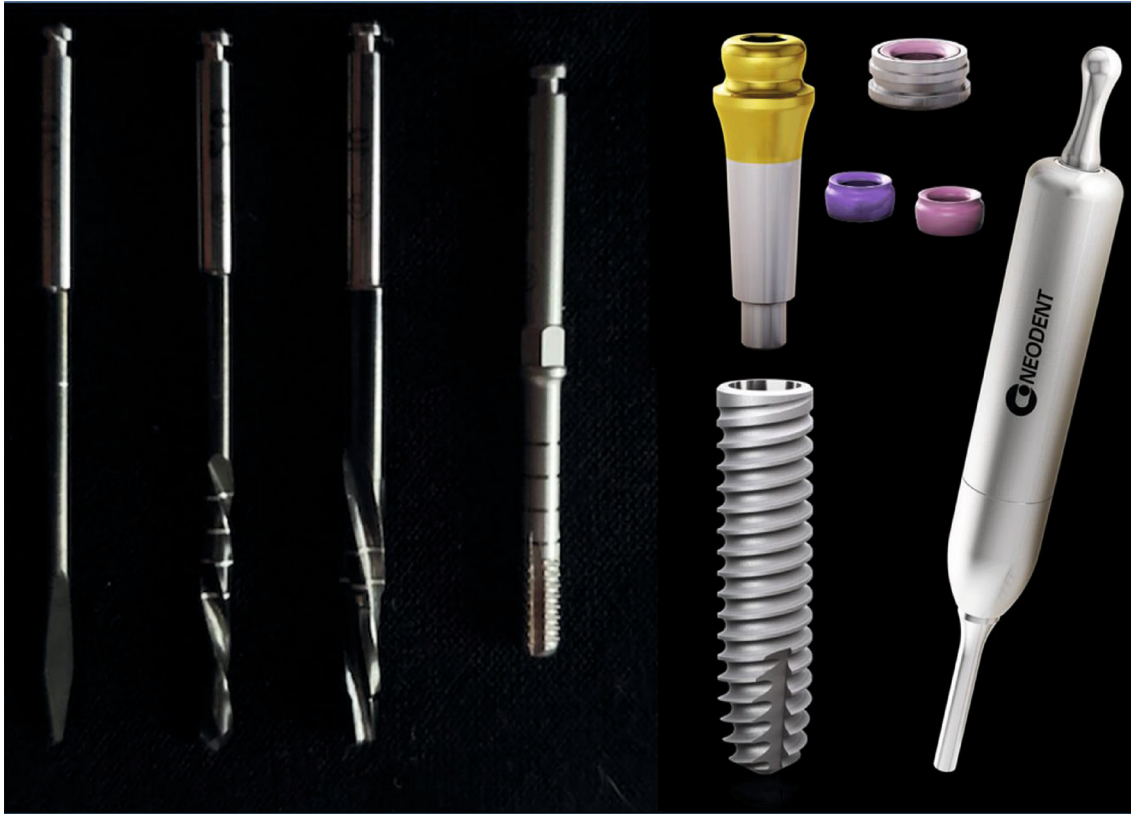
FIGURE 1: The Facility-Equator system. Sequence of drills used for installing the narrow diameter implant (Facility Initial Drill, Facility Twist Drill 2.0, Facility Drill 10, Facility); Facility implant ( \text{\O} 2.9 \text{ mm} \times 10, 12, 14 \text{ mm} ); Facility-Equator attachment, Equator O-ring with Cylinder, Equator O-ring (pink: less retention; purple: more retention), and Facility Abutment Placement Aid.
