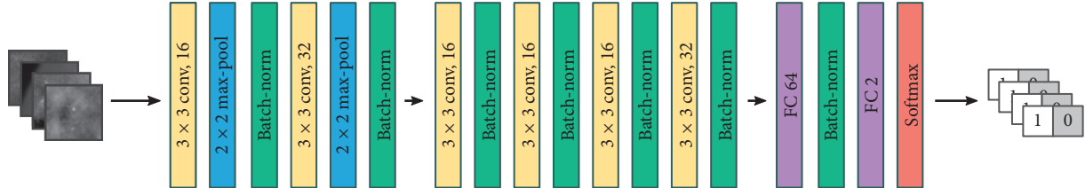
FIGURE 3: Neural network architecture implemented for segmentator and detector.
