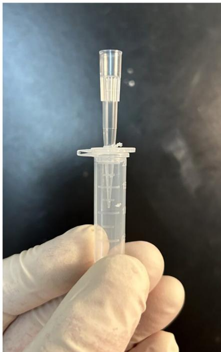
**Figure 8.** A D200 pipette tip with a C<sub>18</sub> plug at the bottom, placed in a 2 mL Eppendorf microcentrifuge tube
