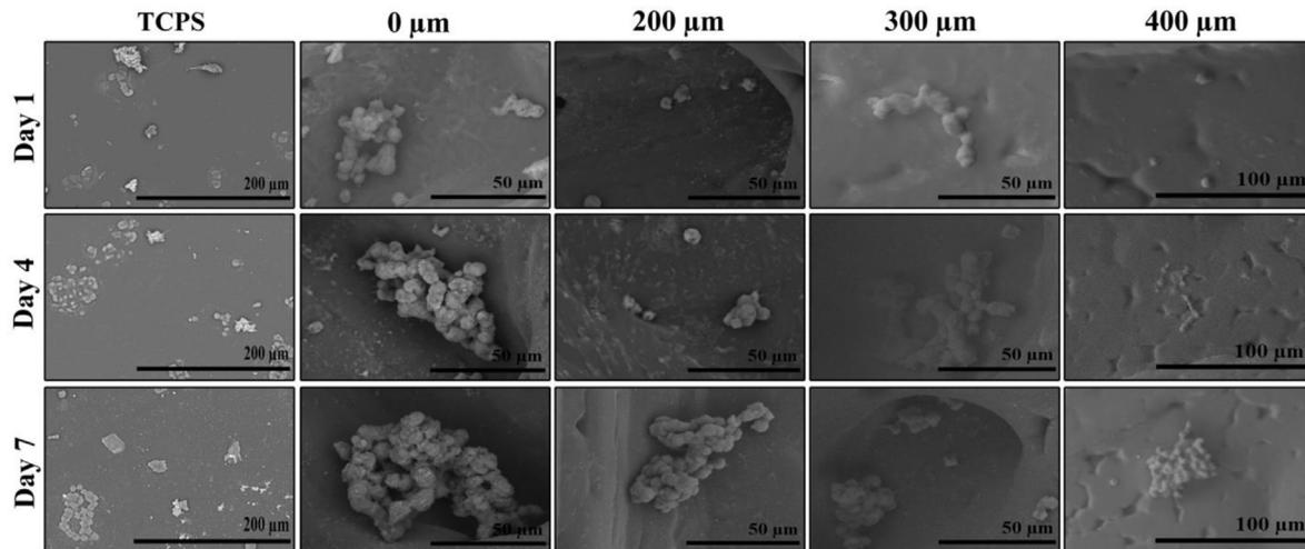
**Fig. 3** SEM analysis for PC12 cell growth morphology and attachment on the PDL (Poly-D-Lysine)-coated TCPS (Tissue culture polystyrene) and PCL (Polycaprolactone) scaffolds with 0, 200, 300, and 400  $\mu\text{m}$  inner diameters of HTA (Half tubular array) at days 1, 4, and 7.
