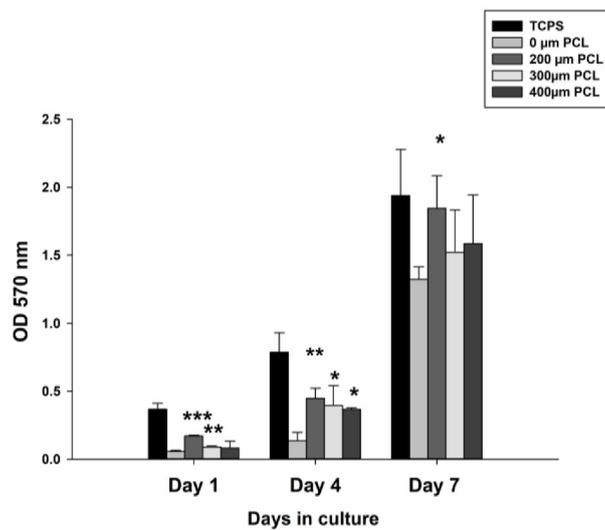
**Fig. 4** MTT assay of PC12 cells on PCL scaffolds with different inner diameters (0, 200, 300, and 400  $\mu\text{m}$ ) of HTA, respectively, 1, 4, and 7 days after cell seeding ( $n = 4$ ). The data are presented as the mean and standard deviation. An asterisk denotes significant differences ( $*P < 0.05$ ,  $**P < 0.01$ ,  $***P < 0.001$ ) in formazan absorbance compared to the PCL scaffolds with a 0  $\mu\text{m}$  inner diameter of HTA. PCL: Polycaprolactone; HTA: Half tubular array.
