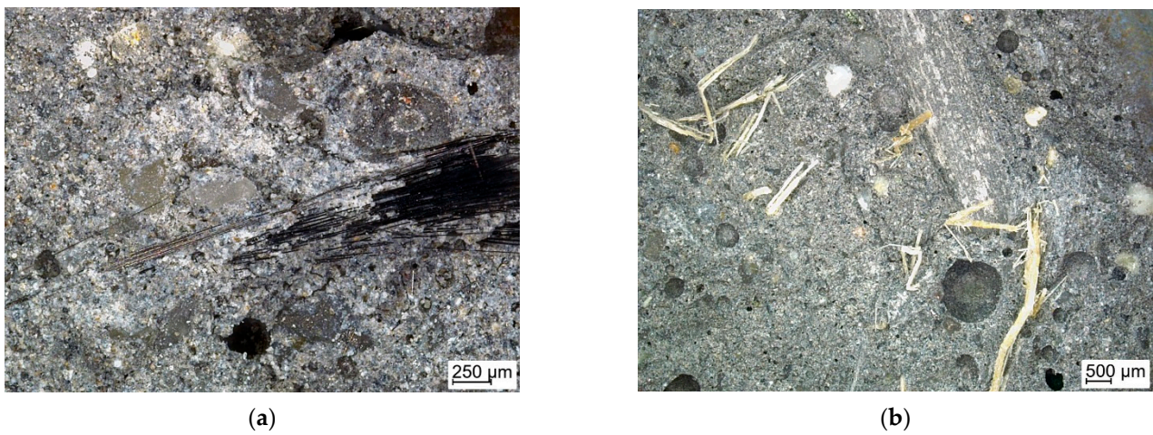
Figure 6. Structure of the composites reinforced with: (a) carbon fiber; (b) flax fiber.
