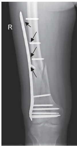
Fig. 2. A 76-year-old man with distal femoral fracture was managed with indirect reduction and submuscular LISS plating. Screw breakage shown on radiograph 9 months postoperatively (black arrows).
