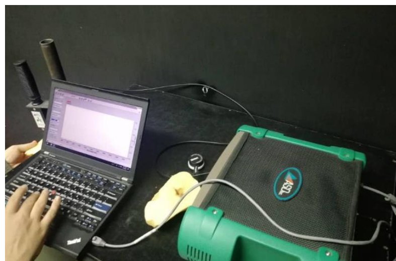
Figure 3. Hardware configuration for obtaining spectral data of the potato samples.
