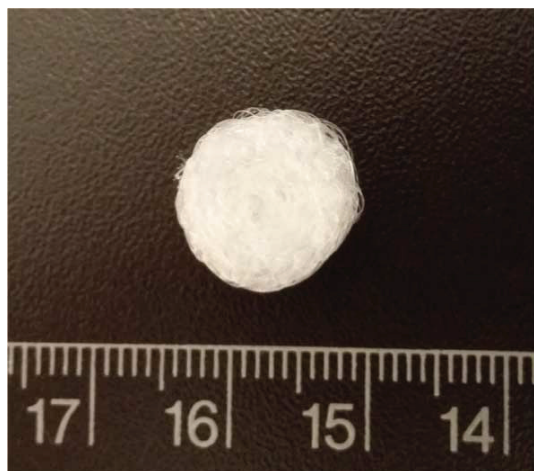
FIGURE 1: A representative image of a knitted 3D scaffold.
