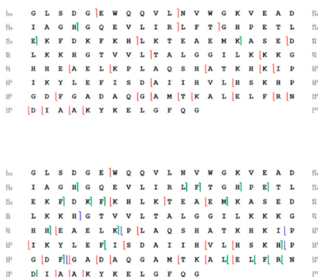
Figure 28. Comparison of ETD (top) and UVPD (bottom) fragmentation used for high resolution top-down HDX-MS. Each notch in the sequence represents a fragment ion that was observable for HDX-MS. Reproduced with permission from ref 257. Copyright 2018 American Chemical Society.
