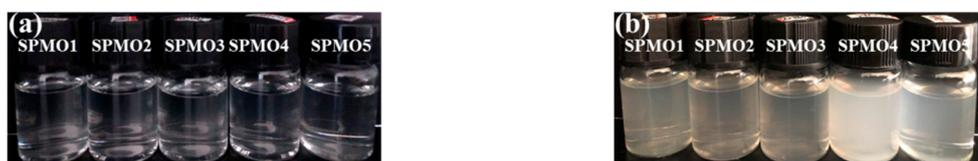
**Figure 4.** Photos of the triblock copolymers aqueous solutions (1 mg/mL) at (a) 25 °C and (b) 35 °C.
