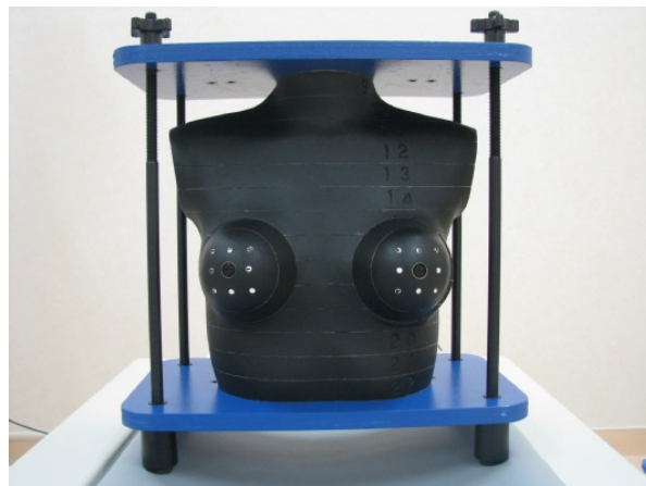
FIG. 1. The anthropomorphic female thoracic phantom used in our study. The entire phantom was cut into thin transverse sections having grids of holes for placement of small dosimeters.
